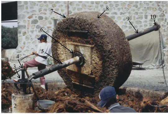
Figure 1. Parts of a Chilean or flour mill: 1 Grinding stone; 2 Rod; 3 Joint; 4 Central axis; 5 and 9 Arm; 6 Arm-wheel union; 7 Stone wheel; 8 Profile; 10 Hauling point.
